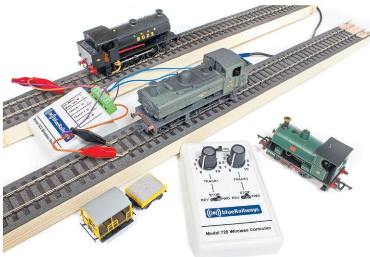
Models as small as the Hornby 'Peckett' and the Bachmann 'Wickham' trolley performed well with the blueRailways' control system. The Model 522 receiver may be programmed in the same manner as the Model 601 using the app to change CVs such as start voltage and maximum speed.
