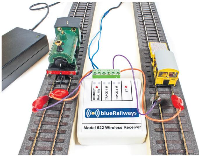
The two track outputs can be wired into a layout with block sections which allow two-train 'cab control' operation using switching to power each block from either one. Common rail return is not recommended for this type of controller because there is only one power source for both track outputs.
