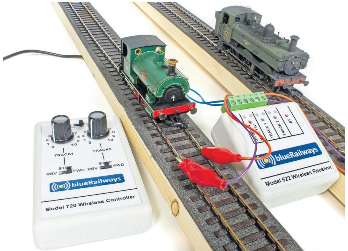
Simple testing of the Model 522 and Model 720 combination using a variety of models. All ran smoothly on the Pulse Width Modulation power output.
