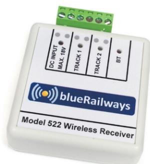
The system is based around a wireless receiver that will communicate with a dedicated handset or mobile devices. This is the Model 522 which is a twin-track receiver.
