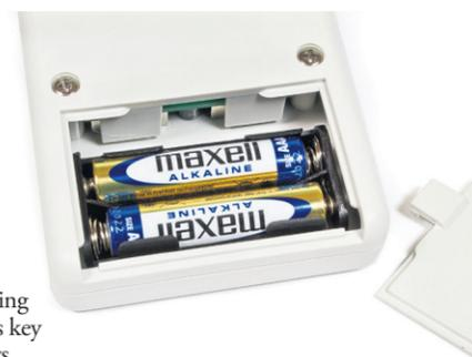
Battery power is usually an issue with wireless controllers because there is no connection to the layout for a source of power. The Model 720 is designed to be very economical with power and battery life can be as long as 1000 hours. The handset has an on-off switch to conserve power between operating sessions.
